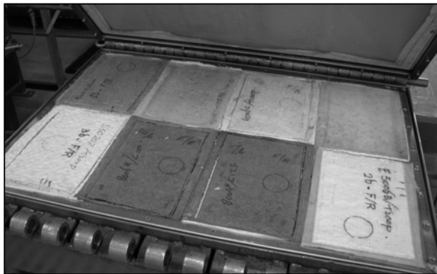
Figure 1. Compressive creep test box
